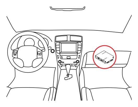
Securely mount and install the interface in a location free from heat, humidity, moving parts, or direct sunlight. Beware of hot-air flow from your vehicle's climate control system. The interface should be secured in a suitable location, free of sharp metal edges, using double-sided tape, Velcro, or wire ties. The adapter's operating temperature range is -30°C to +70°C (-24°F to +158°F)
